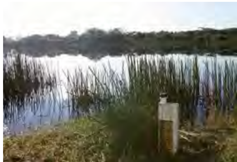
Water level recorder at Lake Serpentine East. Photo courtesy of Environment Waikato.
