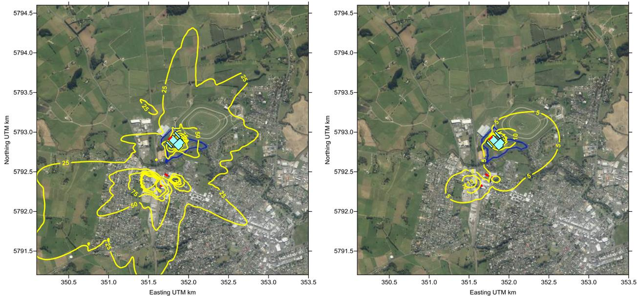
**Figure 6-11.** Maximum long term Nitrogen Oxides  $\mu\text{g m}^{-3}$  (NOx as  $\text{NO}_2$ ) for the RDF plus Fonterra plants. Left panel, 24-hr averages. Right panel annual averages.
