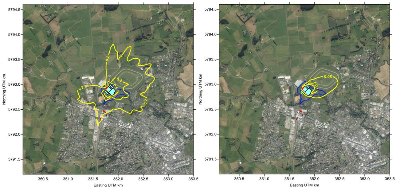
**Figure 6-12.** Fluoride levels in  $\mu\text{g m}^{-3}$  Left panel is for 12-hr averages. Right panel is for 90-day averages
