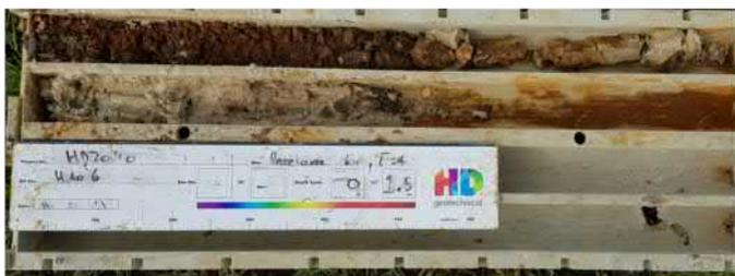
End of auger @ 1.5 m - auger stopped due to no sample retrieval due to high ground water.
