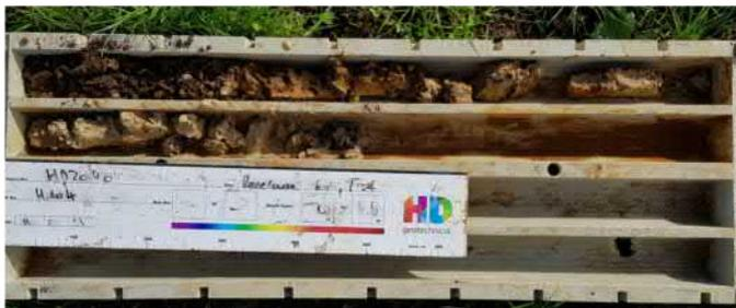
End of auger @ 1.5 m - auger stopped due to no sample retrieval due to high ground water.
