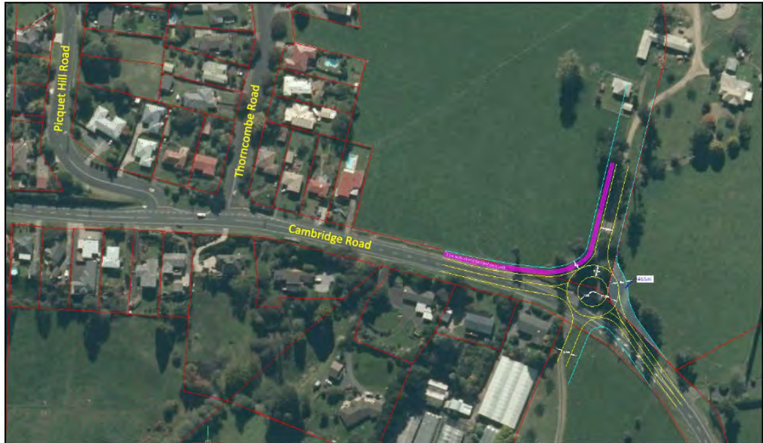
Figure 6. This overlay sketch shows how a roundabout intersection could be situated to provide access to both the T9 cell to the north and the T14 cell to the south
