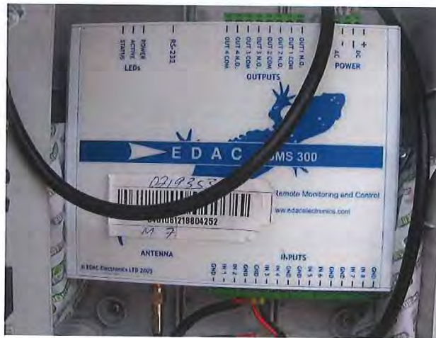
Figure 3. An EDAC SMS 300 dialler unit.
