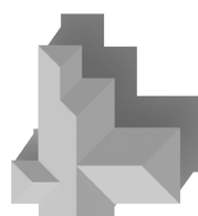
Combination Gable And Hip Roof
