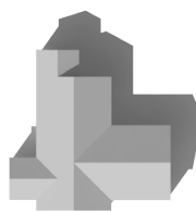
Gable End Roof
