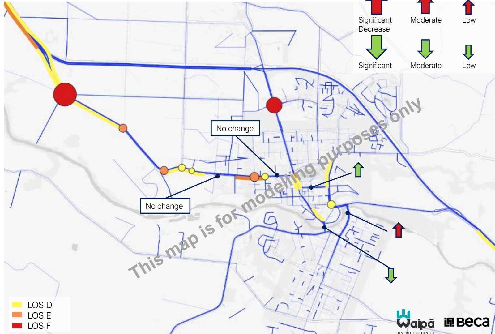
Figure 30: 2055 Option C LOS results and change in traffic volume compared to Do Minimum.
