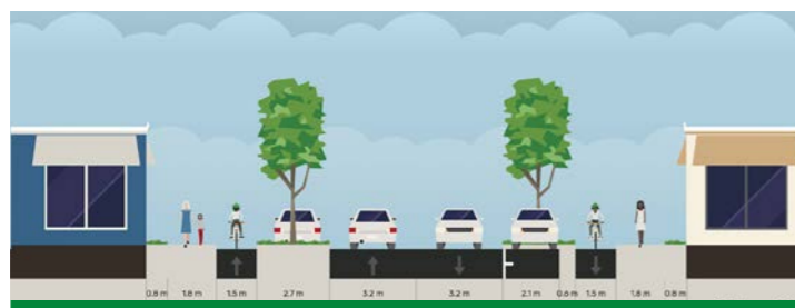
Figure 12. Indicative cross sections
