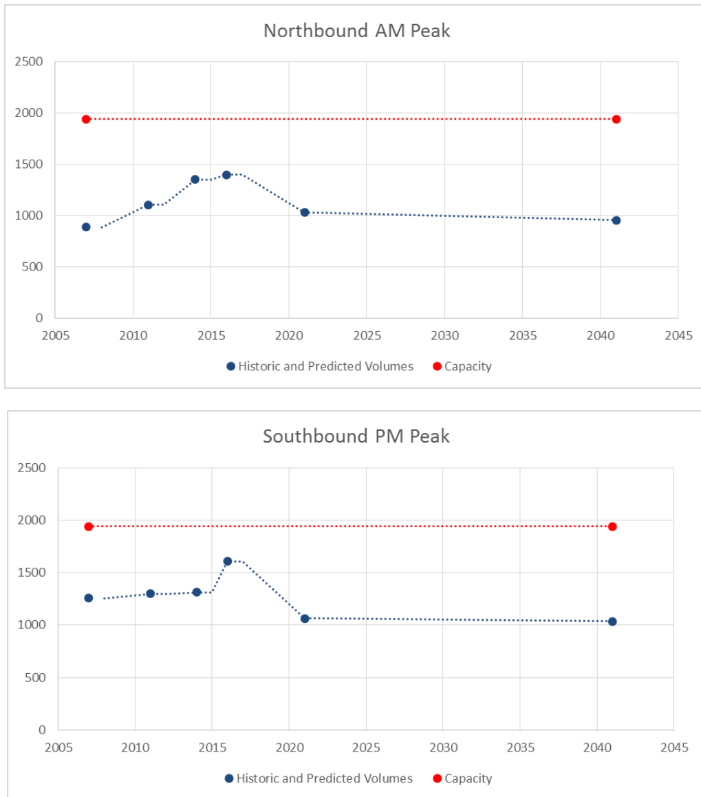
Figure 12: Historic and Predicted Peak Direction Traffic Volumes across Both Bridges Combined
