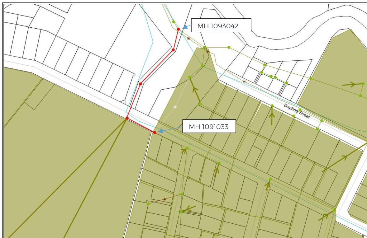
Figure 4 New Pipe Alignment
