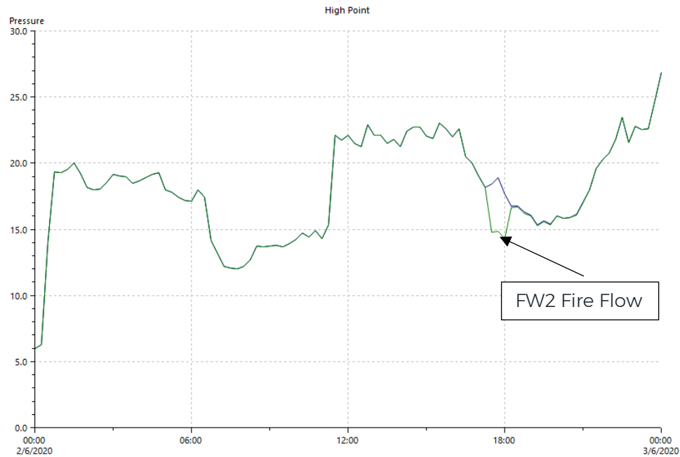
Figure 7. Pressure at high-point within proposed development under FW2 fire flow.
