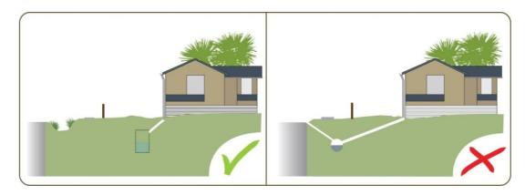
On site detention systems shall ensure that stormwater runoff from the site remains at pre development levels.
