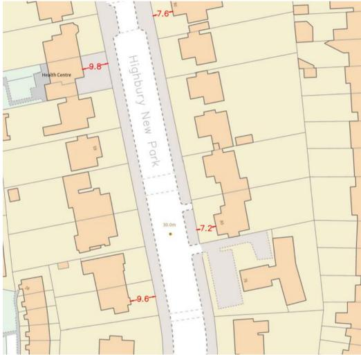
Figure 2: Setback measurements on Highbury New Park, London.
