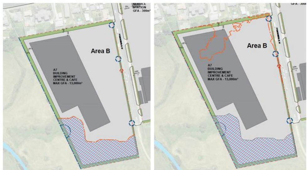
Figure 2: TALFRCP as notified (left), TALFRCP following consultation (right). 1% AEP flood level shown in orange dotted line.
