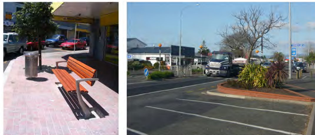
Figure 40: Images of potential streetscape measures including street furniture and landscaping to indicate a slower speed zone at town of Ngatea.
