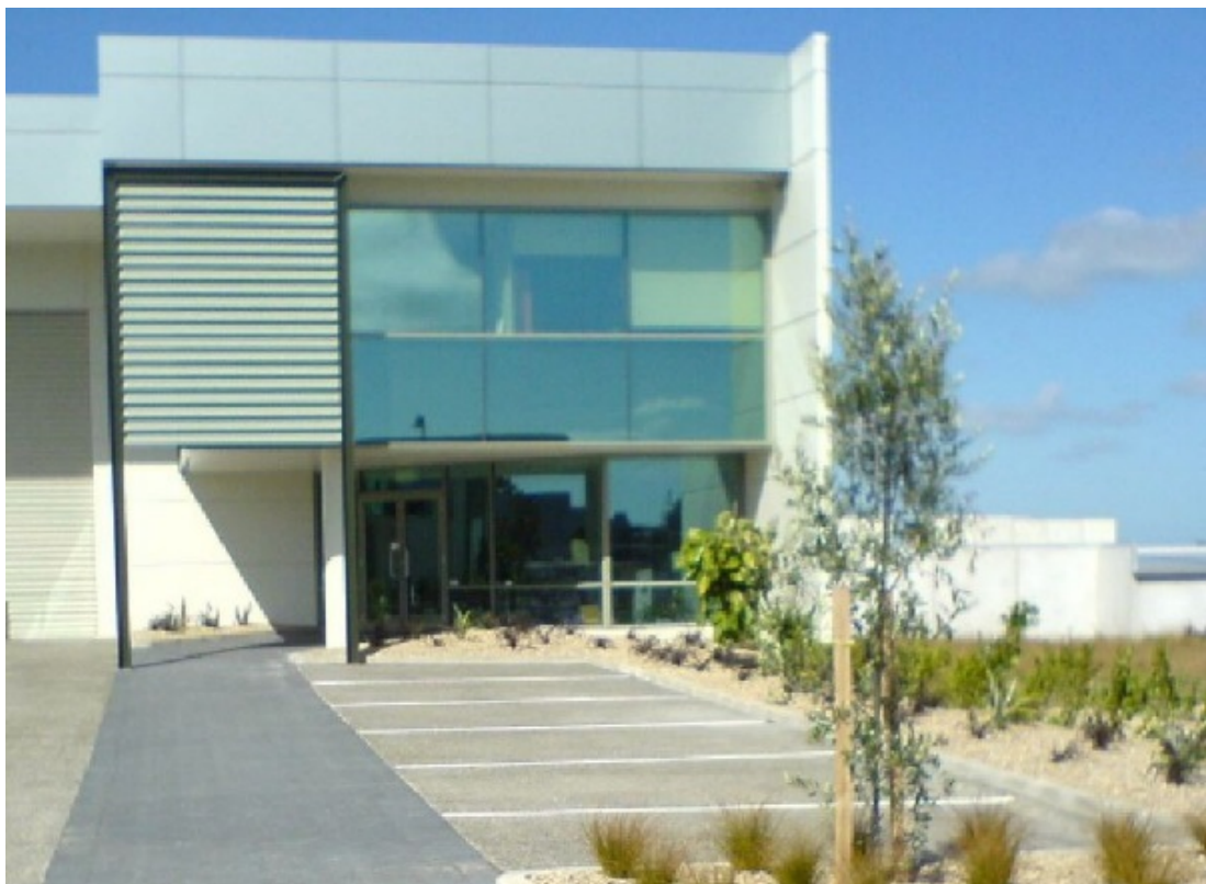
Figure 9 8: A clear and legible front entrance with a glass facade that provides passive surveillance of the car park. A change in surface treatment highlights where the pedestrian footpath leads to the entrance across the car park.
