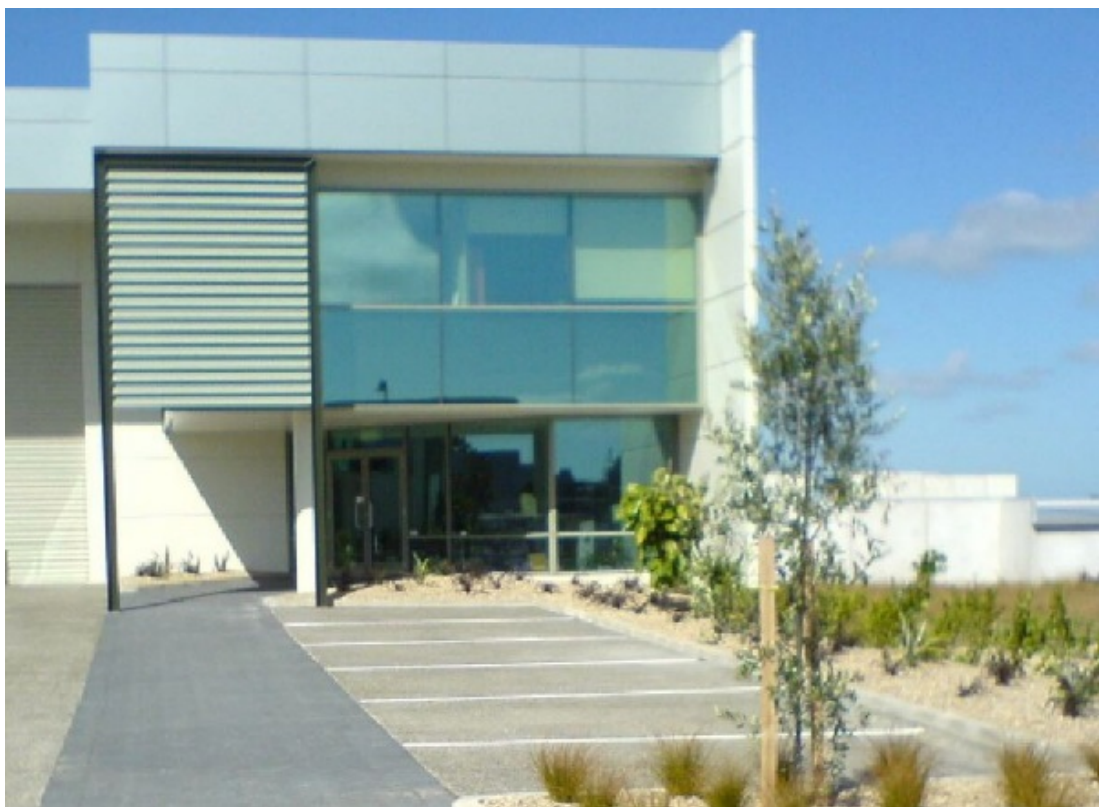
Figure 8: A clear and legible front entrance with a glass facade that provides passive surveillance of the car park. A change in surface treatment highlights where the pedestrian footpath leads to the entrance across the car park.
