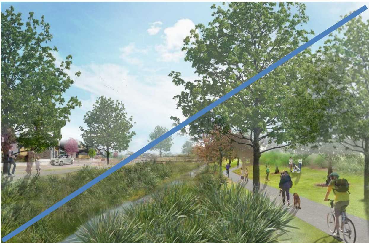
Figure 7: Indicative illustration of the secondary (feeder) stormwater swale within C2 edged by road and housing, with cycle path connections
