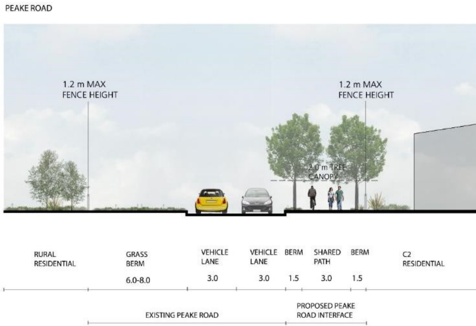
Figure 125: Indicative cross section of Peake Road illustrating the proposed C2 interface
