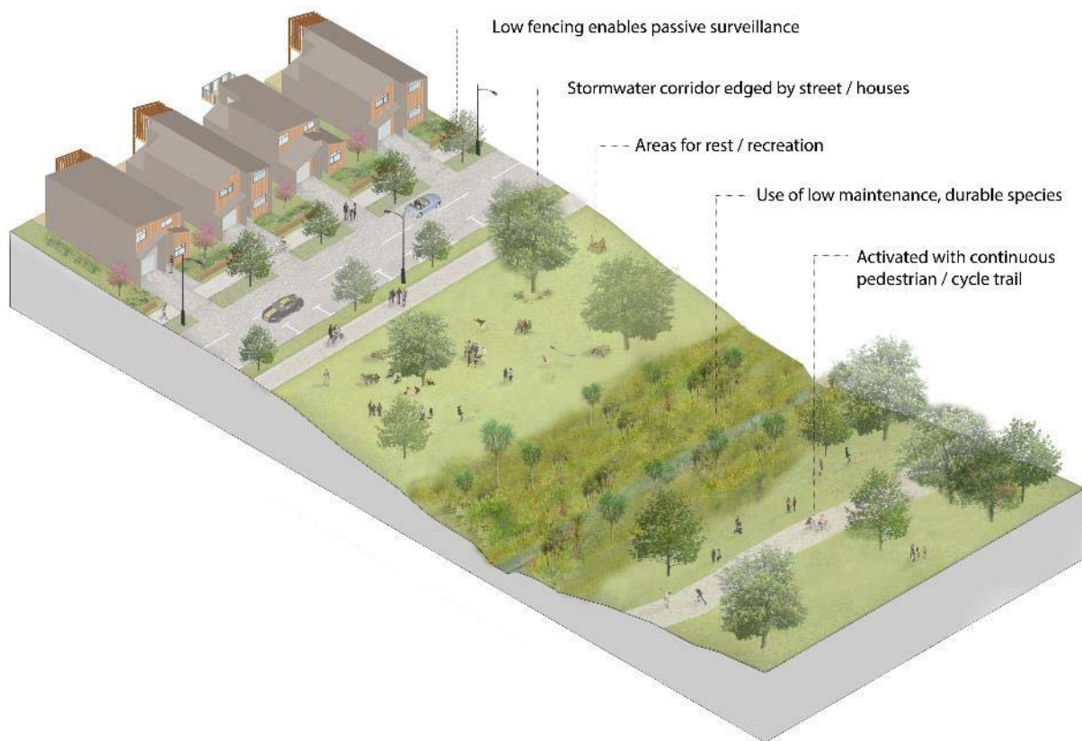
Figure 79: Indicative illustration of the central stormwater swale edged by road and housing, with cycle paths
