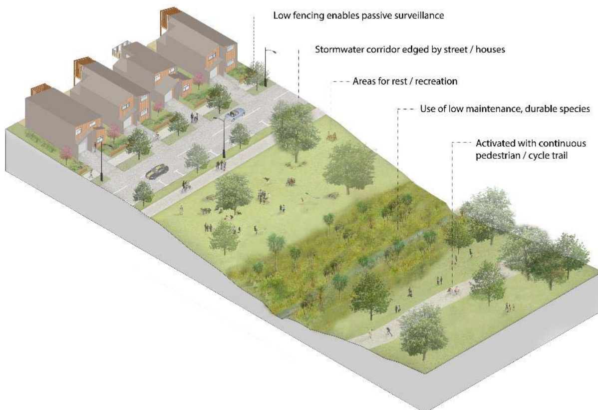
Figure 12: Indicative illustration of the central stormwater swale edged by road and housing, with cycle paths
