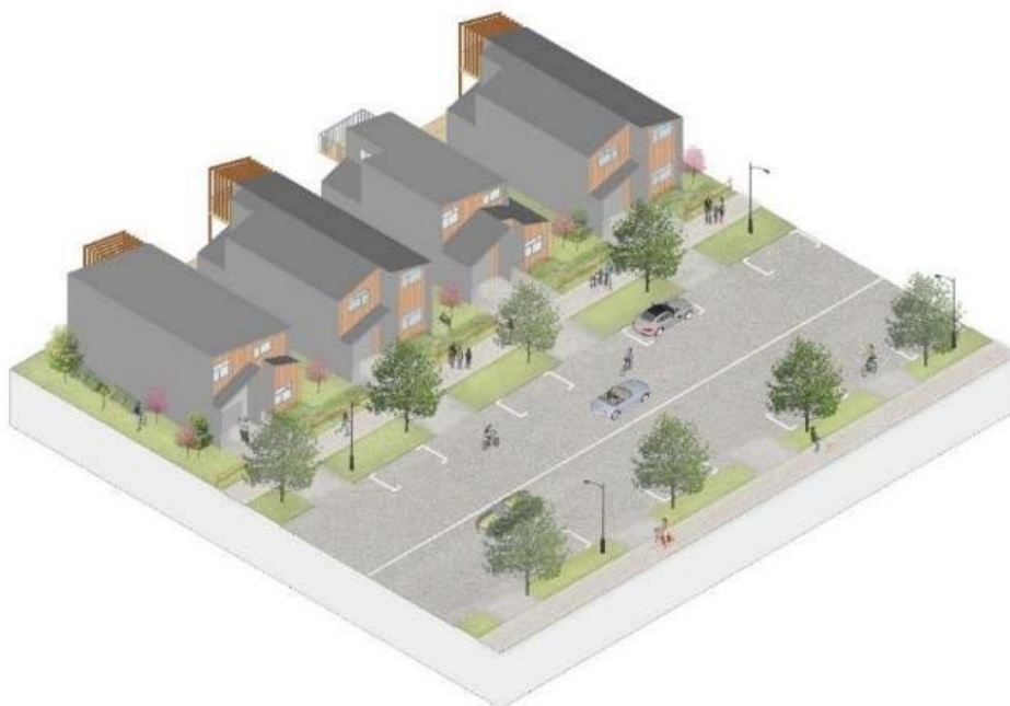
Figure 14: Place street trees at regular intervals, within ample berm space and enable clear sightlines between pedestrians and vehicles
