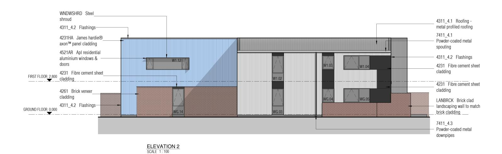
4311\_4.2 Flashings———— 7411\_4.1 Powder-coated metal spouting 7411\_4.3 Powder-coated metal 4521AR Apl residential downpipes aluminium windows & -4851\_4.2 Vertical FIRST FLOOR 2.800 <u>aluminium balustrade</u> 4383 Timber decking-LANBRCK Brick clad 4221AV\_4.2 Vulcan\_ - landscaping wall to match cladding GROUND FLOOR 0.000 \_\_brick cladding\_ \_ \_\_ \_ \_ \_ \_ \_
