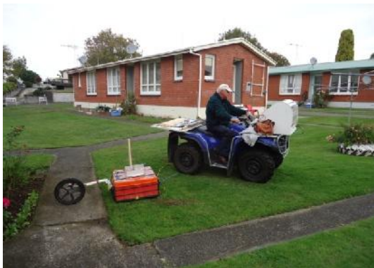
Figure 7 GPR set-up with direct PC readout unit on front of quad
