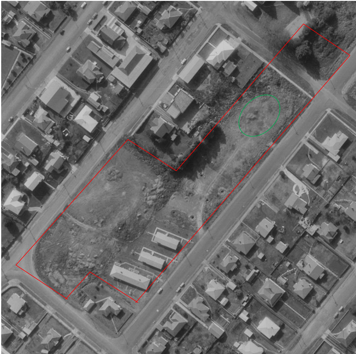
Figure 5 Situation in 1963 (Photo from NZAM). The first 3 retirement homes have been build. All over the site there appear to be stockpiles of materials. Large diameter holes have been drilled north east of the three new buildings. These could have been intended as storm water soak holes. The top NE section seems a natural depression (indicated by the green oval)
