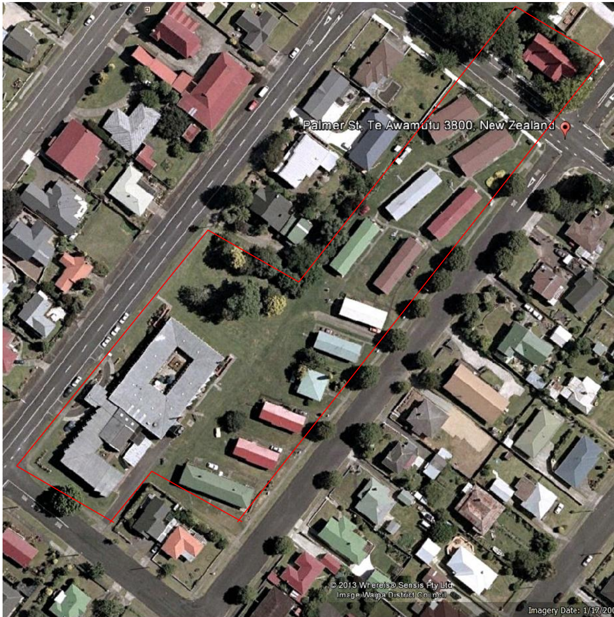
Figure 6 Situation in 2006 Note the community centre (SW corner) is located on a significantly raised area, especially in the NW corner. The building is on a pile foundation and all around the building the ground is subsiding.
