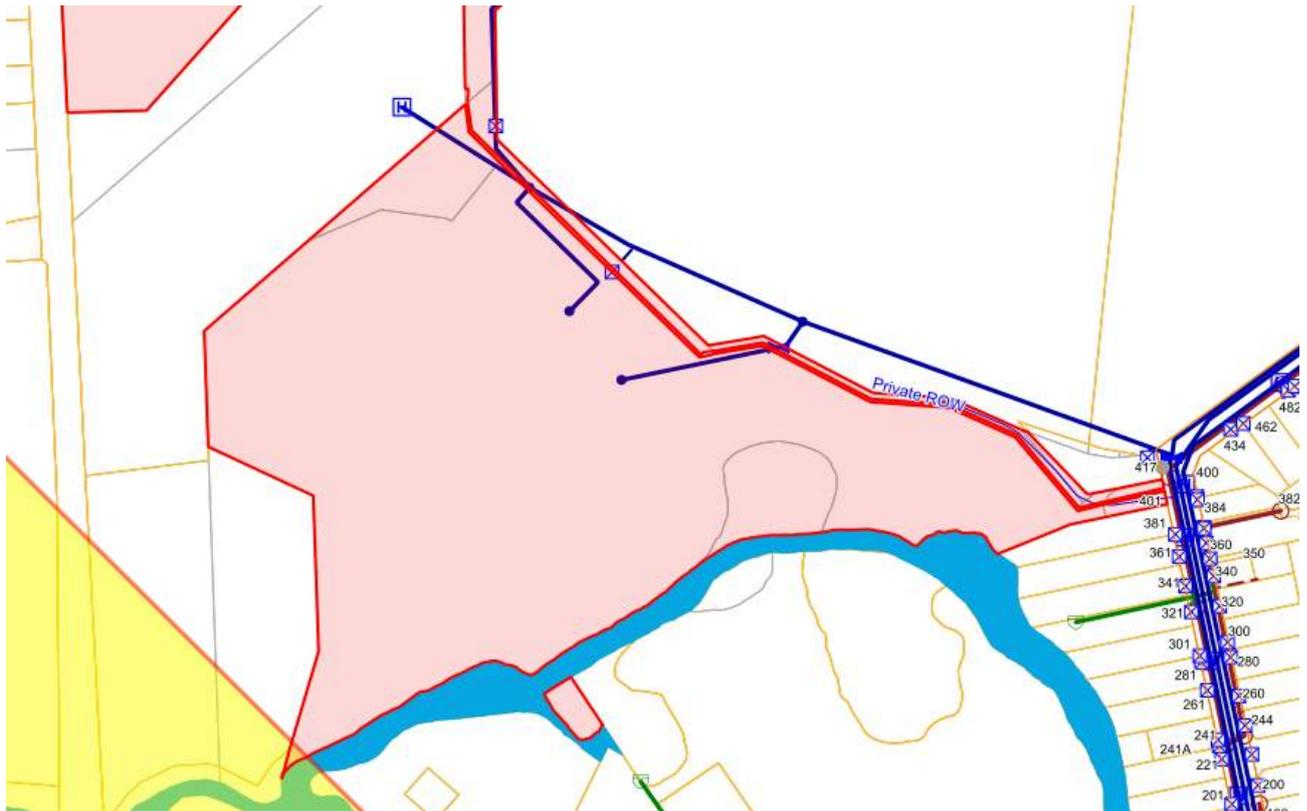
**Figure 4:** Council's Utilities Map (Water supply shown in blue, Stormwater in green, and Wastewater in brown)
