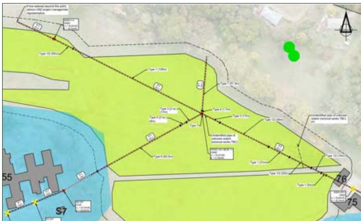
Figure 29: Wastewater demolition plan in Wetland 2
