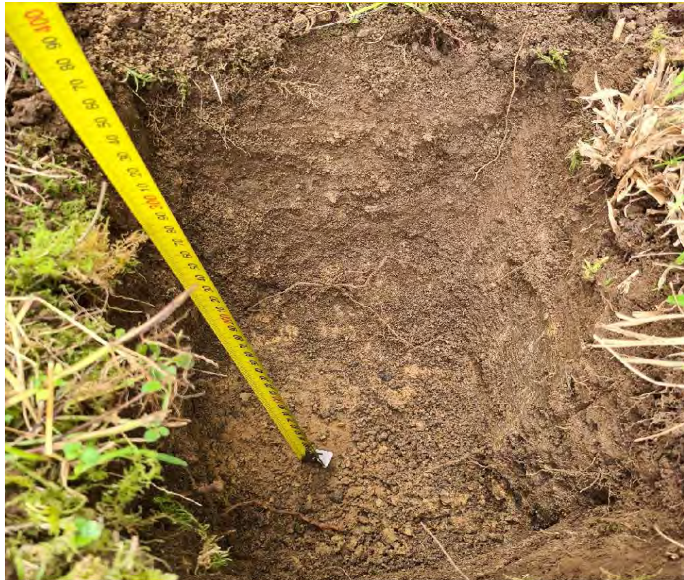
Plate X15: Representative soil profile at B15.
