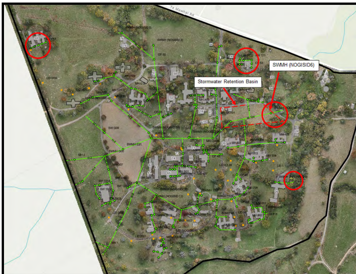
Figure 4 Stormwater discharge points
