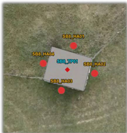
Figure 5 Proposed Asbestos Sampling - Substation 8
