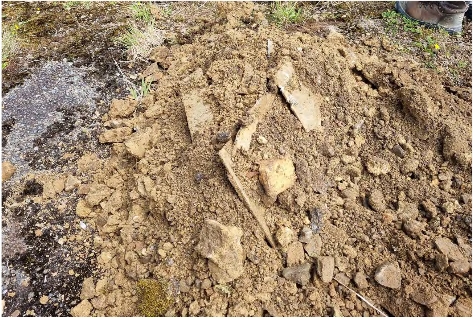
Photo 1 – SB2_TP 03: Asbestos board
