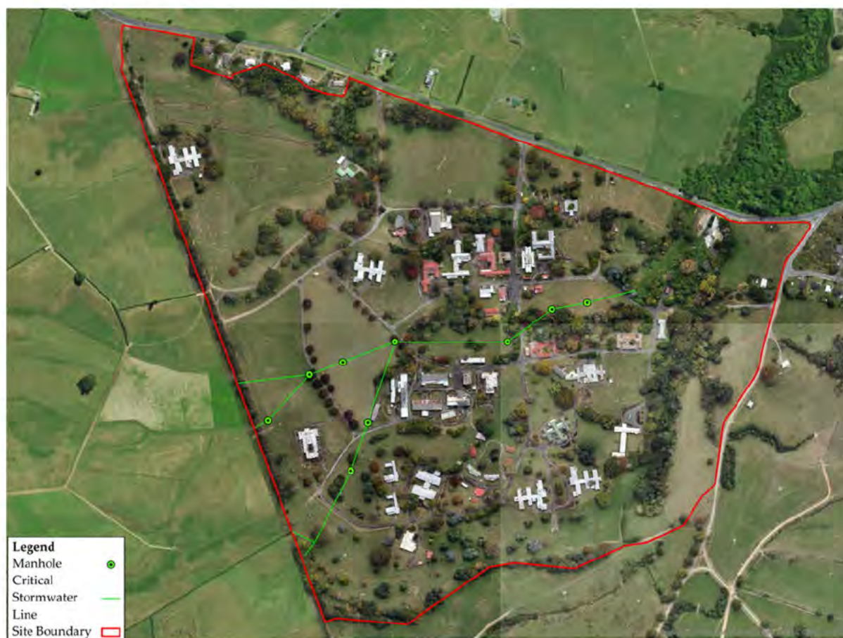
Figure 19: Tokanui Hospital Site – Current Trunk Stormwater Reticulation conveying upgradient runoff through Site
