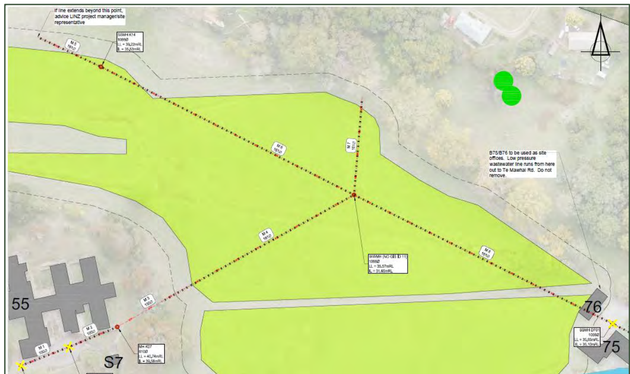
Figure 7: Wastewater lines to be removed within wetland 2 (green area).
