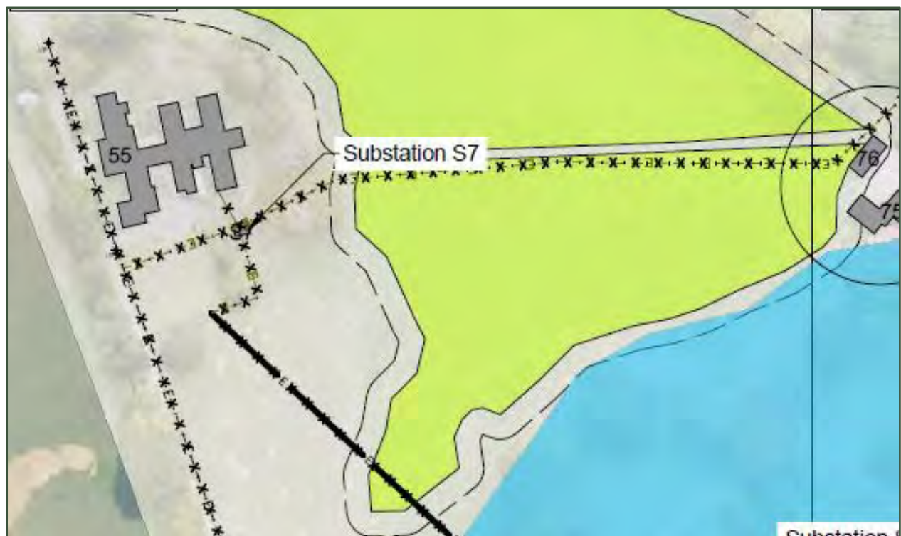
Figure 8: Power line to be removed across wetland 2 (green area).
