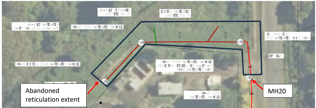
Figure 20: Abandoned wastewater line and MHs (item 13)
