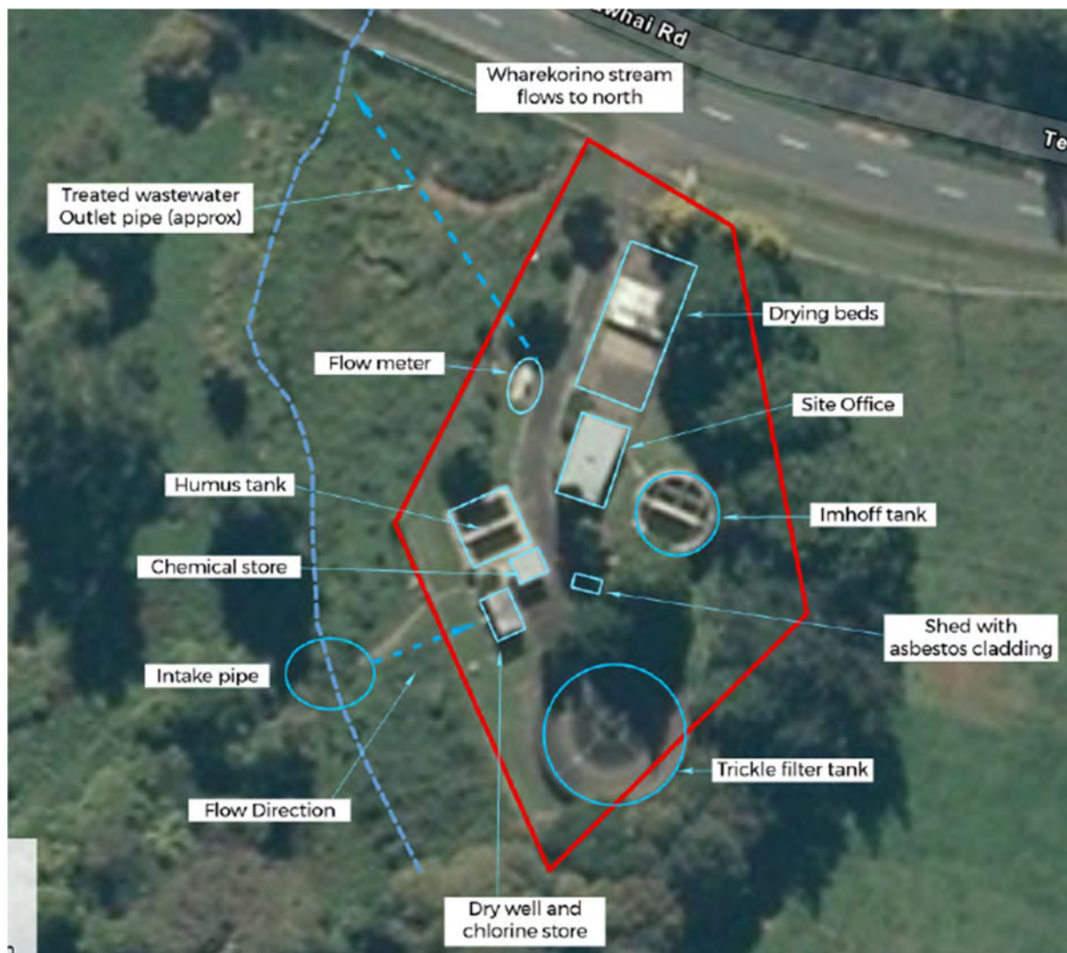
Figure 17: Former WWTP Pre-decommissioning
