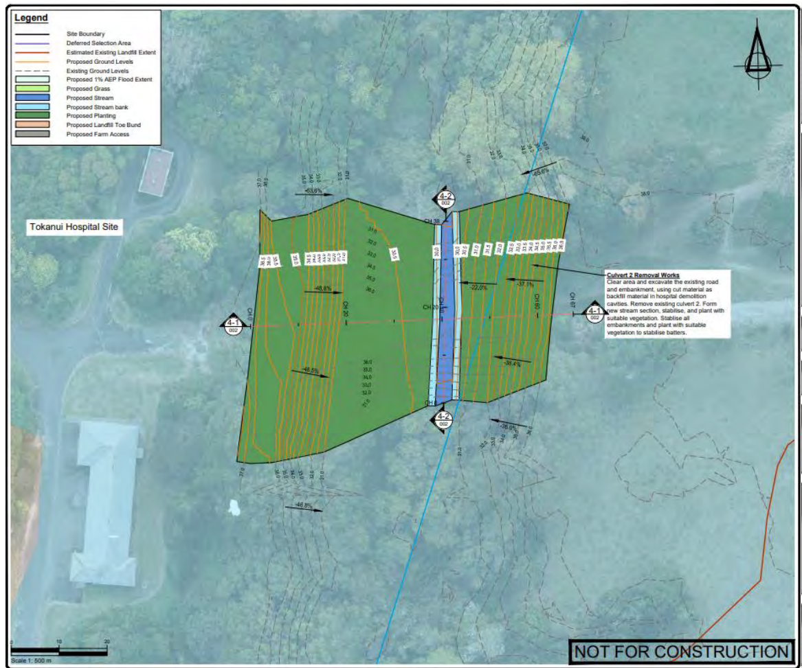
Figure 12: Proposed removal of road embankment and Culvert 2 intersecting the Wharekōrino Stream.
