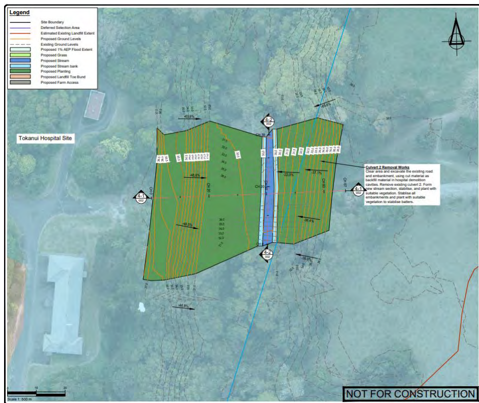
Figure 2: Proposed removal of road embankment and Culvert 2 intersecting the Wharekōrino Stream.
