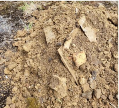
Asbestos cement fragments in soil
