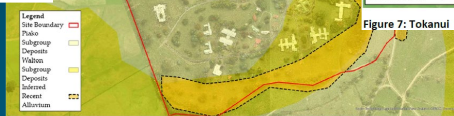
Figure 5: Annotated geological map of Tokanui Hospital site
