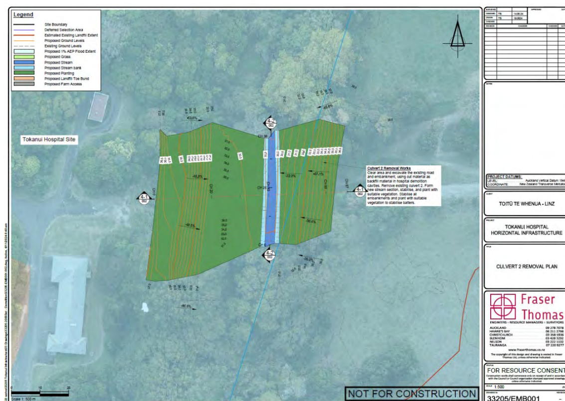
Figure 38: Culvert 2 Removal Plan
