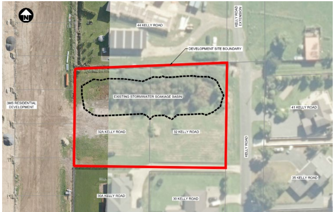
Figure 5. Existing Private Stormwater Soakage Basin at 32 & 32A Kelly Road.
