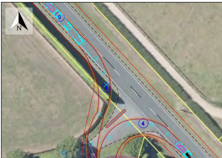
Figure 22: B-train swept paths for entering and exiting vehicle
