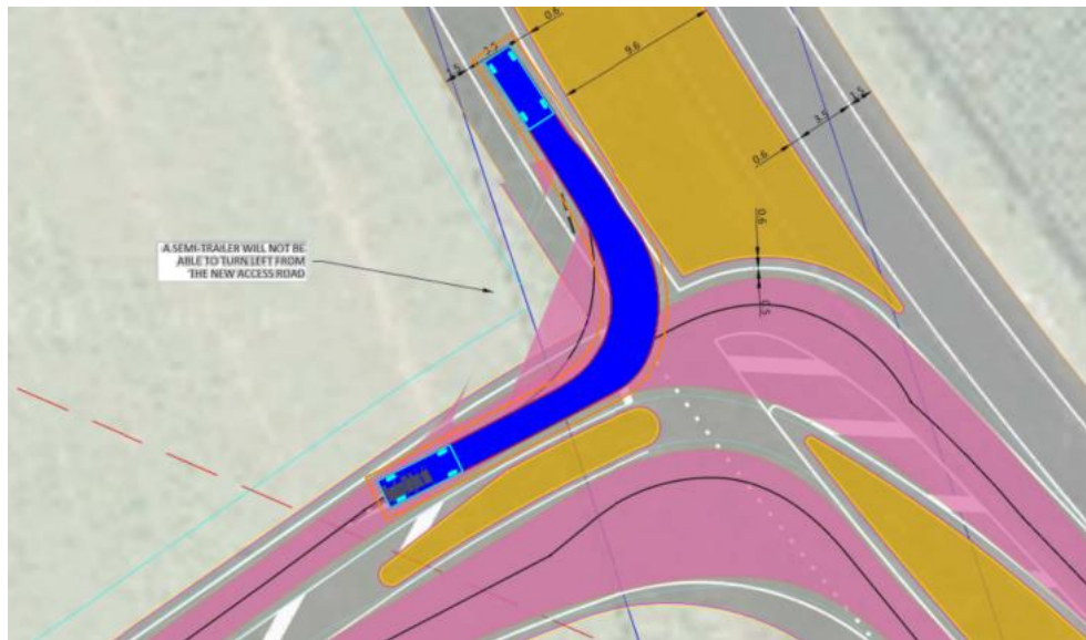
Figure 11: Vehicle tracking indicates 90 percentile car can left-turn
