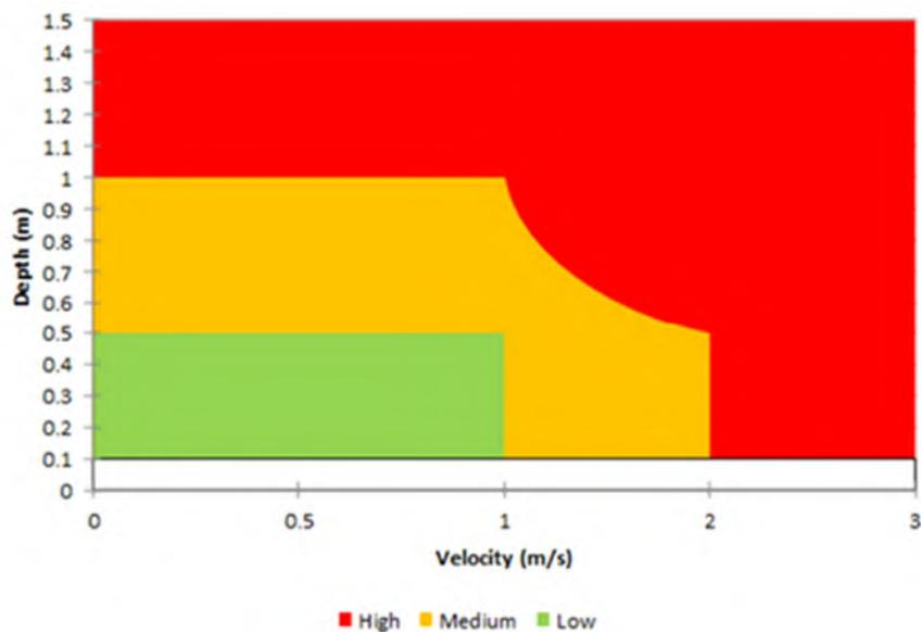
Figure 4. Schematic of adopted Flood Hazard Matrix.
