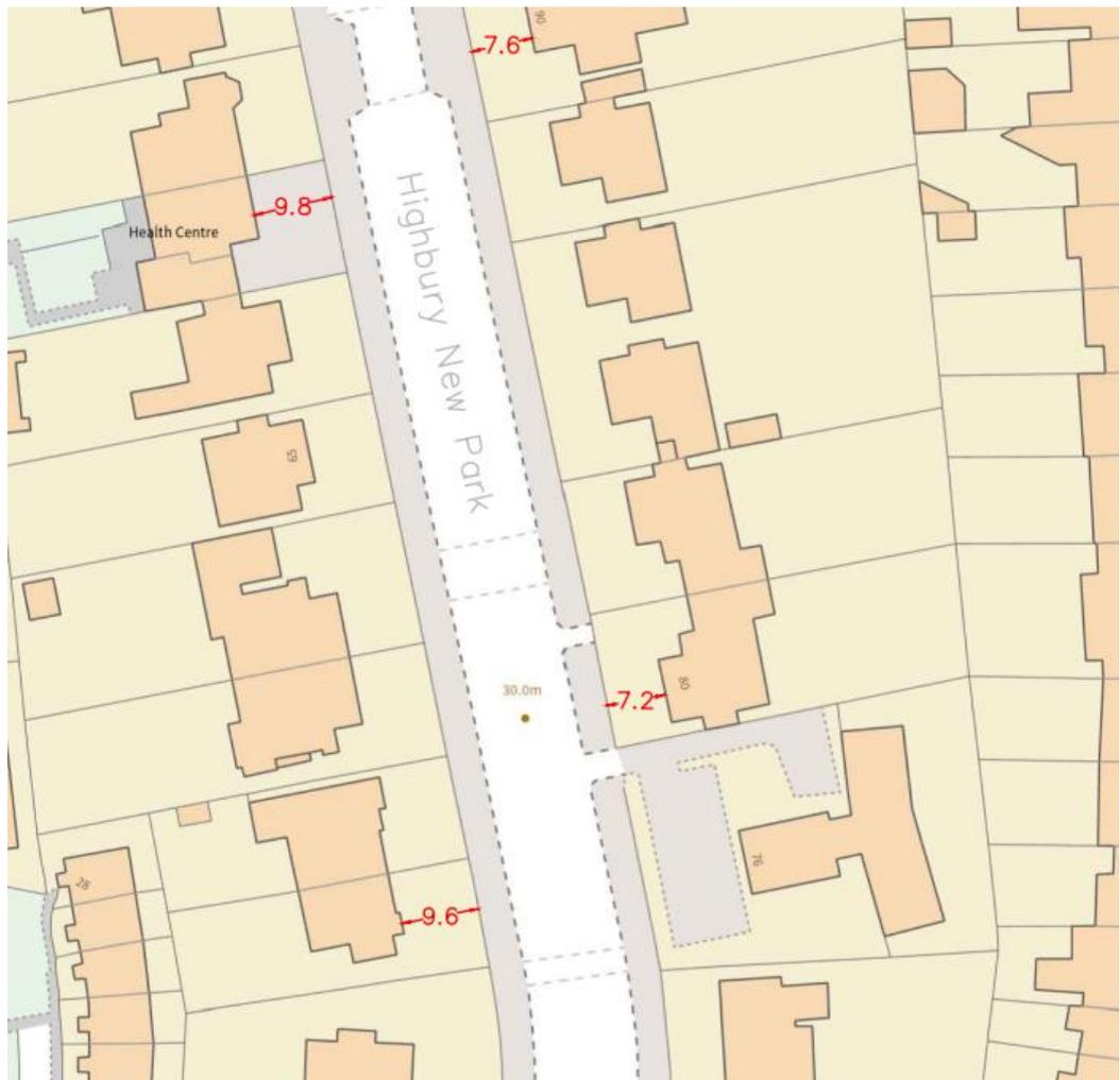
Figure 2: Setback measurements on Highbury New Park, London.
