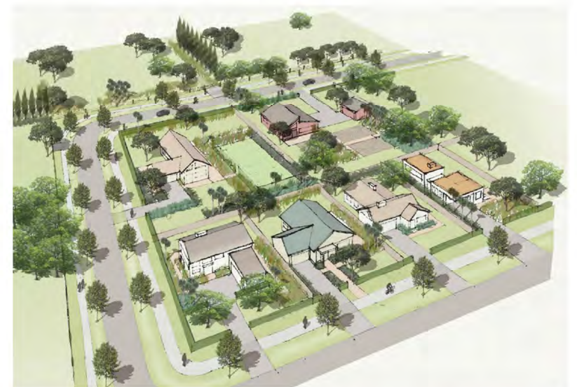
Figure 27: Indicative lot layout, incorporating 1500m 2 lots along the rural interface, and 800m 2 lots internally.
