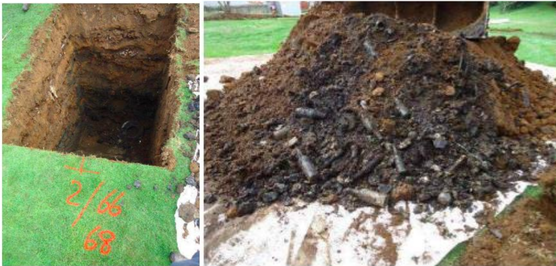
Figure 10 Photograph of environmental testing showing depth of uncontrolled fill and typical artefacts found from the fill layer. Source: AECOM 2015b.
