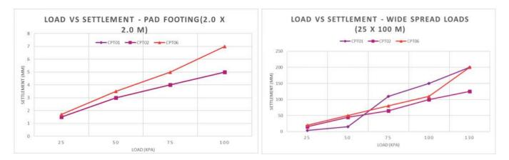
Figure 1: Settlement vs load for a small pad type foundation.
